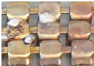
2 Too high temperature
