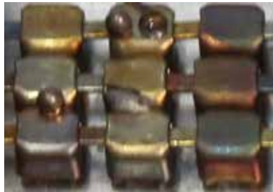
2 Too high temperature
